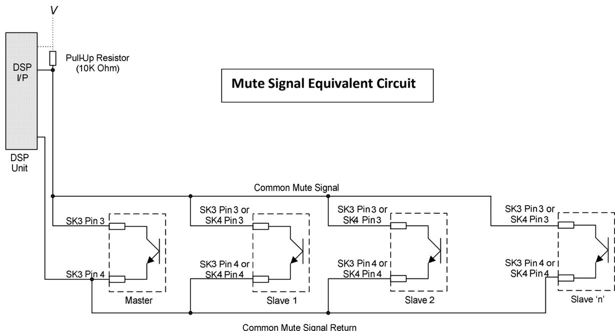
To function correctly, the common mute signal from all units must be connected via an external pull-up resistor (not supplied) to an arbitrary voltage (V) at the DSP as illustrated above. The arbitrary pull-up voltage (e.g. 5V DC or 12V DC) can either be supplied by the DSP itself (preferred option), or by an external voltage source, although if an external voltage source is used, the 0V return must be common with the DSP 0V.
