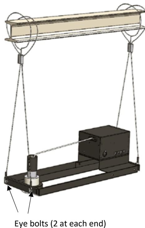
14. Push the free end of the cable harness through one of the holes located on the Gripper. Now loop the free end of the cable over a secure fixing such as a ceiling truss, eye bolt, or any structure capable of taking 7Kgs of weight. Now pass the cable through the remaining hole in the Gripper and then pull on the cable to adjust / take up the slack. Do the same with the other Y cable at the other end of the ceiling tile bracket.
