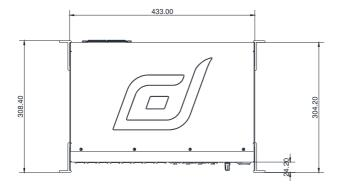
CDM48 - without box Width - 481.6mm/19" Depth - 309mm/12.2" Height - 310mm/12.2"/7U Weight - 12kg/26.4lbs
