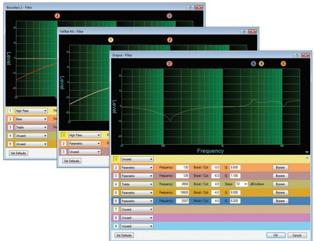
The Filter block offers five customizable filters for each input, three for each virtual bus, and nine for each of the outputs. Each of these filters can be selected as parametric EQ, low pass, high pass, or bass and treble shelving. Standard parameters include frequency, roll-off slope, boost/cut, and Q, depending on the specific filter.
