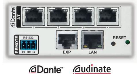
A network with Dante enabled devices can be shared with ordinary data traffic such as e-mail. Audio channels can be transported as unicast or multicast to make the most efficient use of available bandwidth.
