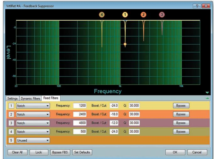
The FBS - Feedback Suppression Block is used to counteract ringing due to frequencies cycling out of control through the microphone and speakers. The feedback suppression processor for the DMP 128 engages up to twenty notch filters with adjustable Q. Fifteen of the filters are dynamic, and the processor automatically detects and then reduces the ringing. Five additional fixed filters can be adjusted manually or transferred from the dynamic filters.
