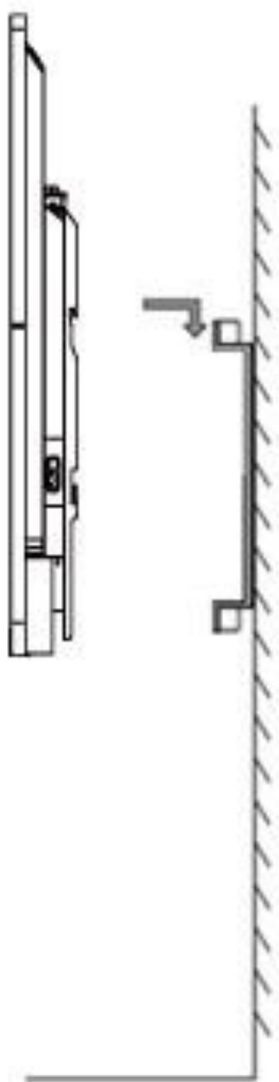
The rear should be installed on the hook holes
