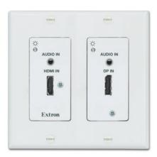
The Extron DTP T DWP 4K 332 D is a decorator-style transmitter that provides signal extension for up to two sources, sending DisplayPort or HDMI, audio, and control up to 330 feet (100 meters) over a shielded CATx cable to Extron DTP™ 330-enabled products. The HDCP-compliant transmitter includes several integrator-friendly features in a convenient form factor that offers maximum placement flexibility.
