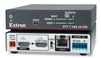
The Extron DTP T HD2 4K 230 transmitter sends HDMI with embedded audio, plus bidirectional control signals up to 230 feet (70 meters) over a shielded CATx cable to Extron DTP®-enabled products. The HDCP-compliant transmitter includes several integrator-friendly features that streamline installation. Its compact enclosure enables discreet installation in a wide variety of applications.
