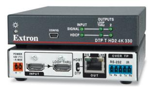
The Extron DTP T HD2 4K 330 transmitter sends HDMI with embedded audio, plus bidirectional control signals up to 330 feet (100 meters) over a shielded CATx cable to Extron DTP® 330-enabled products. The HDCP-compliant transmitter includes several integrator-friendly features that streamline installation. Its compact enclosure enables discreet installation in a wide variety of applications.
