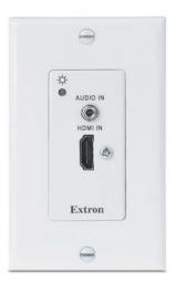
The Extron DTP T HWP 4K 331 D is a single-gang decorator-style transmitter for sending HDMI, analog audio, and bidirectional control signals up to 330 feet (100 meters) over a shielded CATx cable to Extron DTP™ 330-enabled products. It is designed for efficient use within configurable rooms and environments offering limited space. The HDCP-compliant transmitter features a convenient one-gang form factor that offers maximum placement flexibility.
