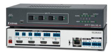
The Extron DTP T SW4 HD 4K is a four-input switcher with a DTP output that sends HDMI and control signals up to 330 feet (100 meters) over a shielded CATx cable. With integrator-friendly features in a compact enclosure, this switcher is well-suited for a variety of applications.
