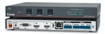
The Extron DTP T USW 333 switcher provides signal extension for up to three sources, sending HDMI or analog video, audio, and control up to 330 feet (100 meters) over a shielded CATx cable to Extron DTP® 330-enabled products. The HDCP-compliant switcher includes several integrator-friendly features in a low profile enclosure that enables discreet installation in a wide variety of applications.
