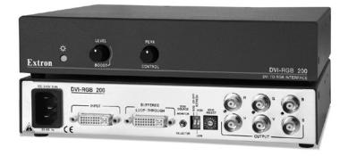
The Extron DVI-RGB 200 converts single link DVI-D signals to analog RGB signals. It is ideal for integrating digital video sources into conventional analog-based A/V systems. The DVI-RGB 200 is equipped with several convenient features for integration including EDID Minder, a buffered DVI input loop-through, and variable level and peaking controls for the analog RGB output.
