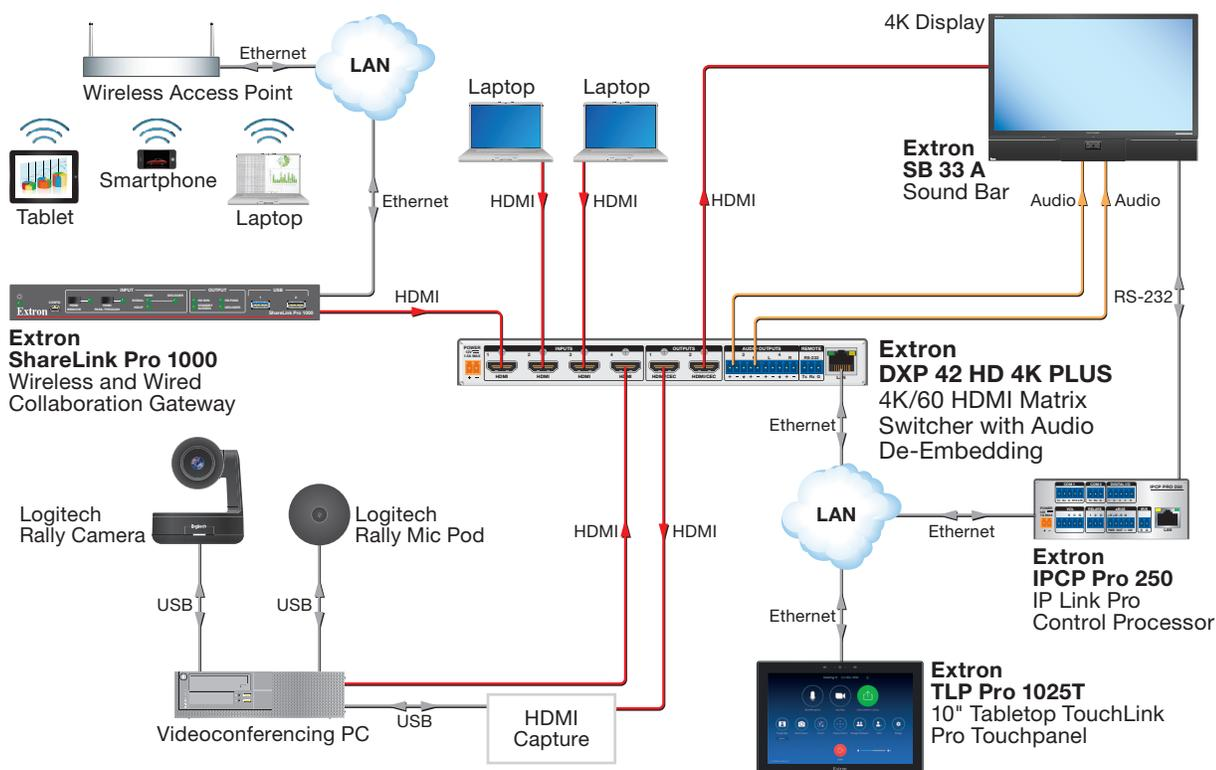
Figure 1. Typical Application of the DXP 42 HD 4K PLUS
