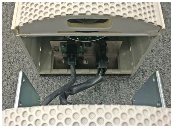
Make connections and slide the modules together
