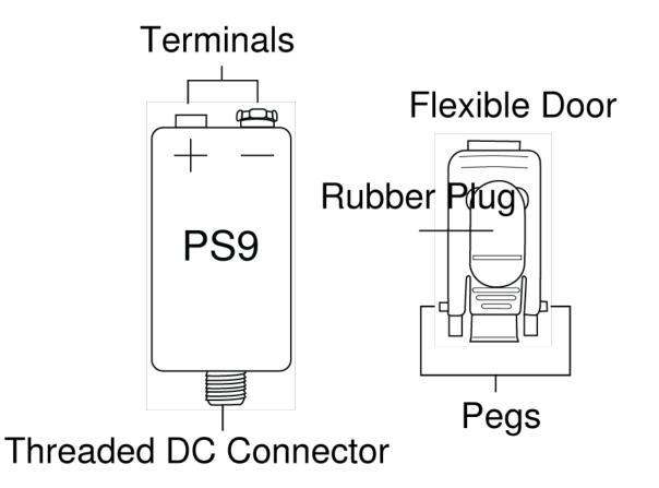
The PS9 takes the place of a 9V battery, allowing you to connect a PS4 AC adaptor to the following Shure bodypack receivers and transmitters:
