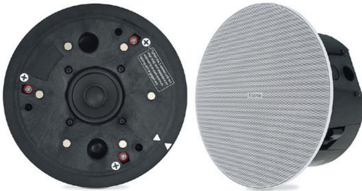
The Extron SF 3C LP is a full-range ceiling speaker featuring a 4" deep low profile composite back can. The redesigned 3" (7.6 cm) full-range driver features a wider and smoother frequency range of 65 Hz to 20 kHz and is engineered with an extremely wide conical dispersion of 165°. The SF 3C LP speaker is ideally suited for small to medium applications with lower ceilings and low to medium power requirements.
