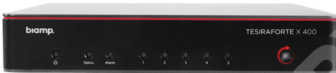
TesiraForte X 400 is a meeting room DSP featuring multiple network and analog audio connection points, with 4 channels of Acoustic Echo Cancellation (AEC) assignable across any digital or analog input. 5 Ethernet ports are provided, four of which are PoE+ powered, and all of which support media and control traffic of various types including AVB, Dante and VoIP.
