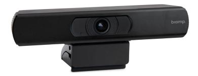
The Vidi 100 is a 4K camera for use with conferencing systems. Intended for huddle rooms or small conference rooms, the Vidi 100 has a 120° wide field-of-view, allowing everyone in the room to be seen. It can be table-mounted or attached to the room's display. The Vidi 100 is also equipped with a microphone array and built-in noise cancelling algorithms to ensure everyone in the room is heard clearly, regardless of where they are sitting or standing.
