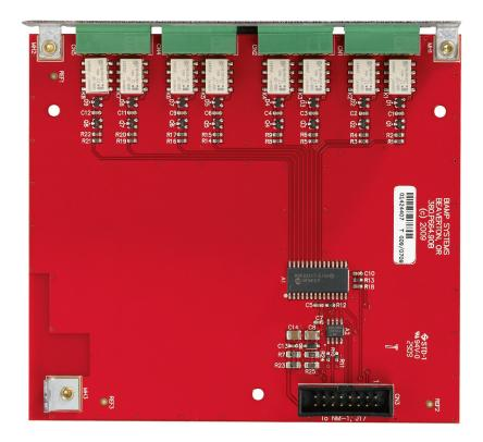
The PARM-1 Page Active Relay Module is an optional module for the VA-8600 amplifier. It provides a SPDT relay contact connection for each VA-8600 amplifier channel (total 8 relays). A relay will be energized when paging is active in the corresponding AM-600 amplifier channel.
